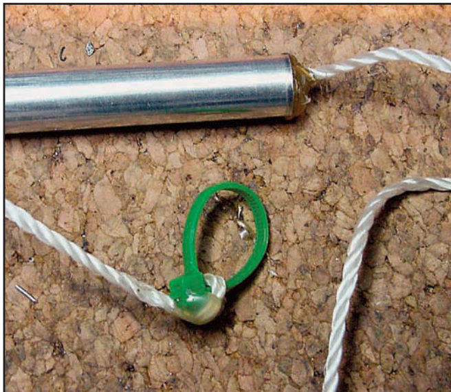
Figure 10—A set of 3 guys was made by using a wire tie (closed to slip over the top of the telescoping whip but not over the base of the whip). Hot glue was used to attach a nylon line to each wire tie. Hot glue was also used to attach the guy line to a left-over length of brass tubing.
