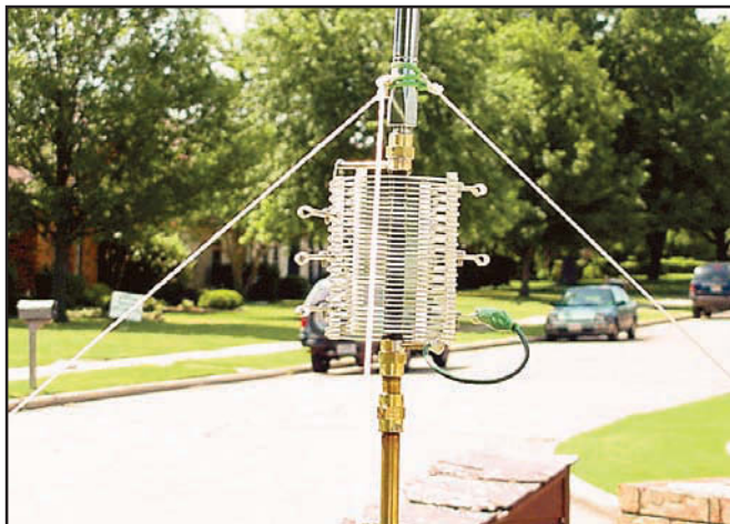
Figure 11—A close-up of the guy lines attached to the telescoping whip. The coil and coil clips detail can also be seen.
