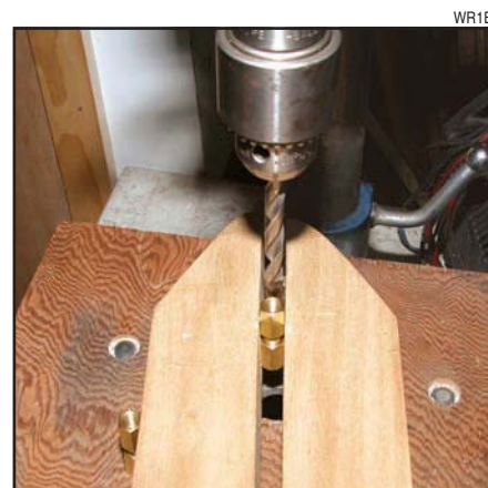
Figure 4—A pipe coupling and nipple secured in a woodworker's clamp ready to drill out the end on a drill press.
