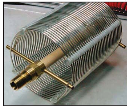
Figure 7—The loading coil assembly ready to be soldered.
