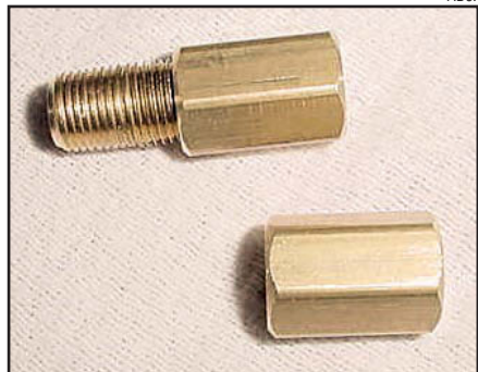
Figure 5—After the pipe couplings have been drilled out and one coupling removed from the nipple, the pair is ready to be installed on the ends of an 18 inch length of brass tubing.
